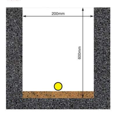
The trench depth must be a minimum depth of 600mm and have a width of at least 200mm, care must be taken to ensure that the backfill material is free of sharp stones or objects that could damage the polyethylene(PE) pipework.
